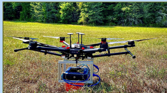
In work done over the summer of 2023 by UNH graduate student Tim Hoheneder , a Ground Penetrating Radar (GPR) antenna was attached to a UAS drone and flown at Thompson Farm Research Observatory. Tim is developing a system to allow for easier measurement of snowpack and soil conditions. His report, and those of other recent UNH Fellows, is available on the NHSGC website.
