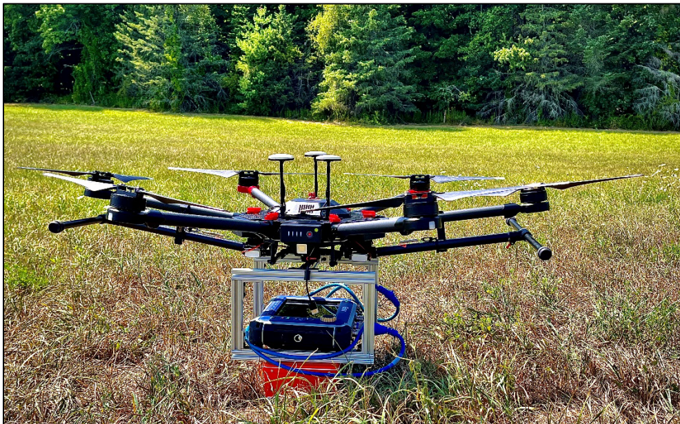
Figure 1: UAS-GPR Platform Consisting of a GSSI 900Hz Ground Penetrating Radar Antenna, GSSI SIR 4000 Controller Unit mounted on a DJI Matrice 600 UAS
